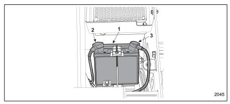
Figure 4-18 Battery and Cable Connections
